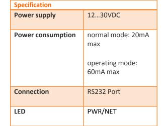
G900i-232 has possibility to connect to PC serial port due to transmission of data or text message. Also connect to some control equipment such as data loggers with RS232 port to manage system. GPRS connectivity makes you have a remote management system that always
